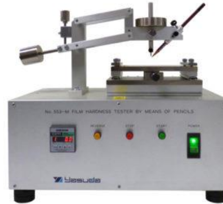
No553 Pencil Scratch Hardness Tester
