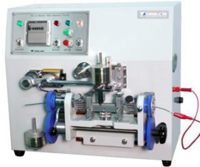
No.210 Magnet Wire Abrasion Tester
