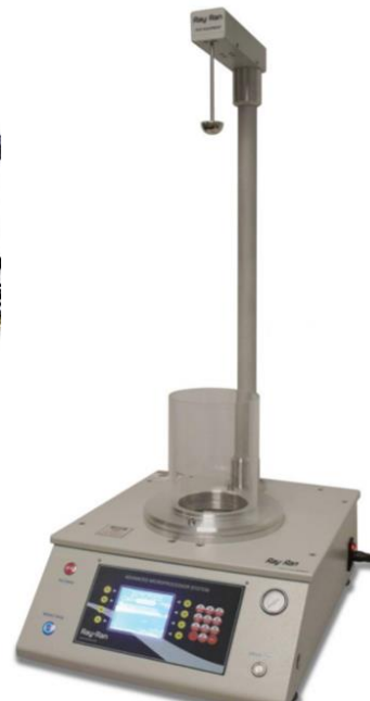
(b) Static spherical indenter (blister test)
