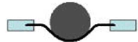
(c) Uniform hydrostatic pressure bulge test
